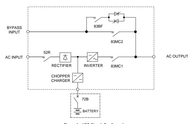
Figure 9 - UPS Circuit Configuration.
